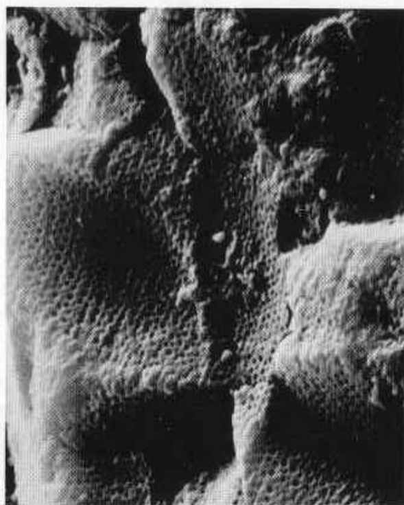
Etched fracture surface of plastic treated Brazilian opal magnified 6,500xs
