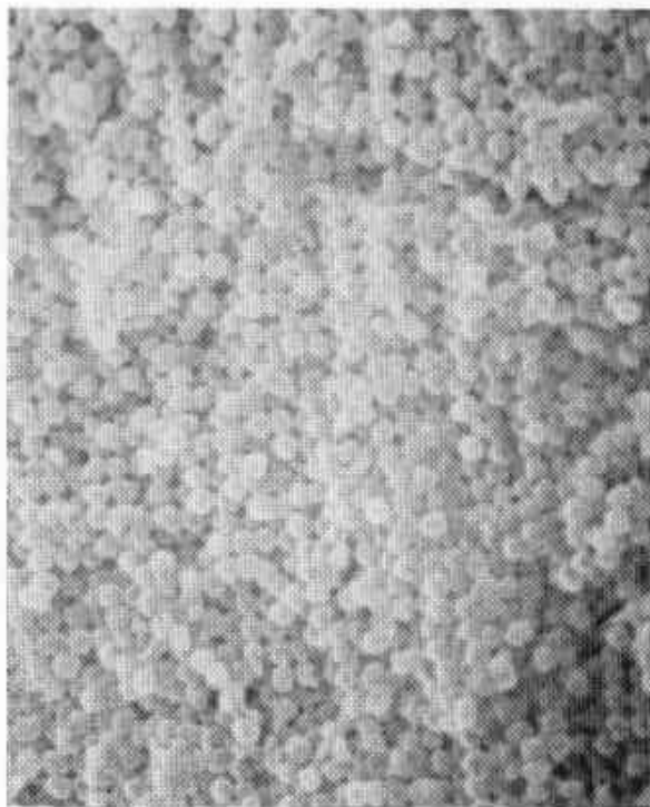
Scanning electron microscope view of etched surface natural Australian opal magnified 14,000xs
