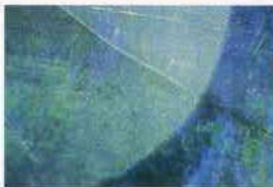
Plastic treated and dyed Brazilian opal showing detail of wisp-like veil of dye along crack and removal of dye in etched area.
