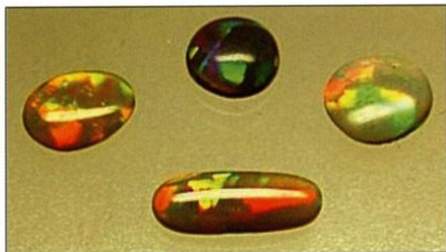
Fig. 18c After soaking in water the hydrophane opal porosity becomes filled and the play of colour becomes more conspicuous, (transmitted light, 10x).
