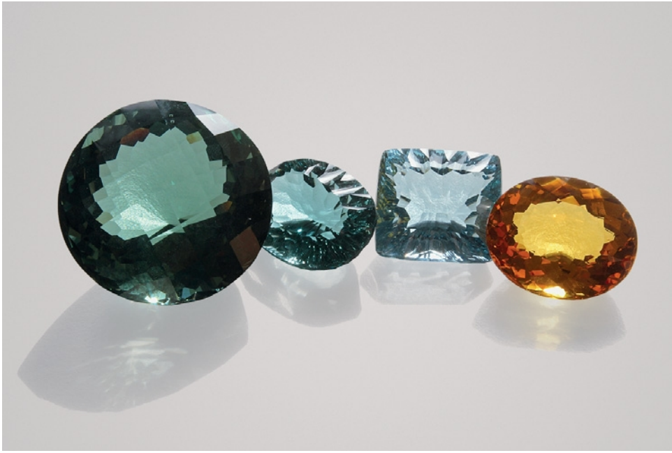
Figure 31. These large faceted samples, submitted as amethyst (even though dark green), aquamarine, and citrine, proved to consist of synthetic quartz. The largest weighs 162 ct. Photo by Evelyne Murer, © Gübelin Gem Lab.
