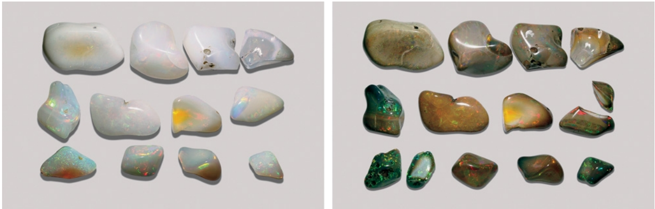
Figure 34. These opals from Wollo, Ethiopia, are shown before (left) and after (right) sugar-acid treatment. Darker bodycolors were produced in samples with a greater hydrophane character. The broken opals (center-right and bottom-left) show the shallow penetration depth of the treatment. The samples measure from 13 \times 9 \times 7 mm (lower right) to 29 \times 16 \times 10 mm (upper left). Photos by F. Mazzero.
