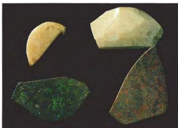
Figure 5. Treatment of different colors of Andamooka matrix opal (top) produces different types of carbonized matrix opal (bottom). Experienced treaters know which types of untreated material will produce the most attractive carbonized opal.
