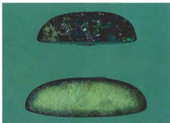
Figure 6. In most cases, the carbon treatment penetrates the matrix opal only at the surface of the prepolyed stone. Here, the chipped surface of the cabochon at top reveals the whitish color of the original matrix opal. Cut lengthwise, the cabochon at the bottom graphically illustrates the relatively shallow depth of penetration of the carbon.
