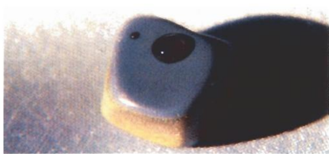
Fig. 14. Photograph of a single Russian 'silica' 'synthetic' opal bead showing the absorption of a drop of water, the nature of the grey 'potch' surface, and indistinct columnar nature of the colour 'grains' or patches. Specimen courtesy of Manfred Zsykora.
